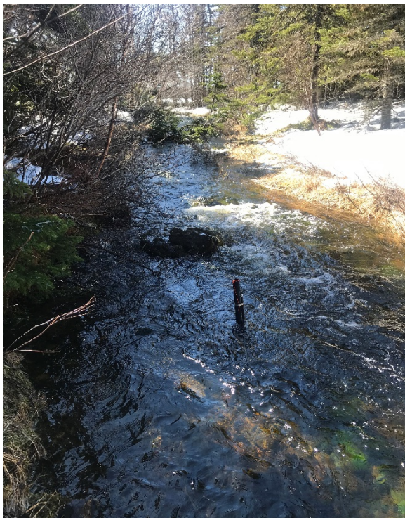
Figure 3-1: Pressure transducer installed in Great Pond Outflow
